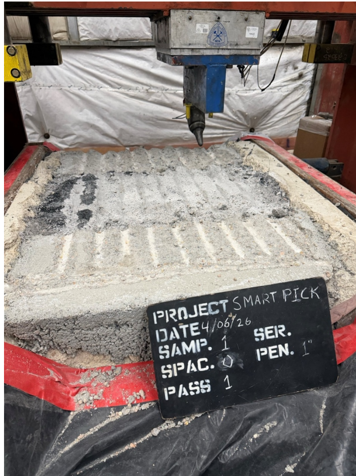
Figure 32 Rock Specimen After Several Passes.
