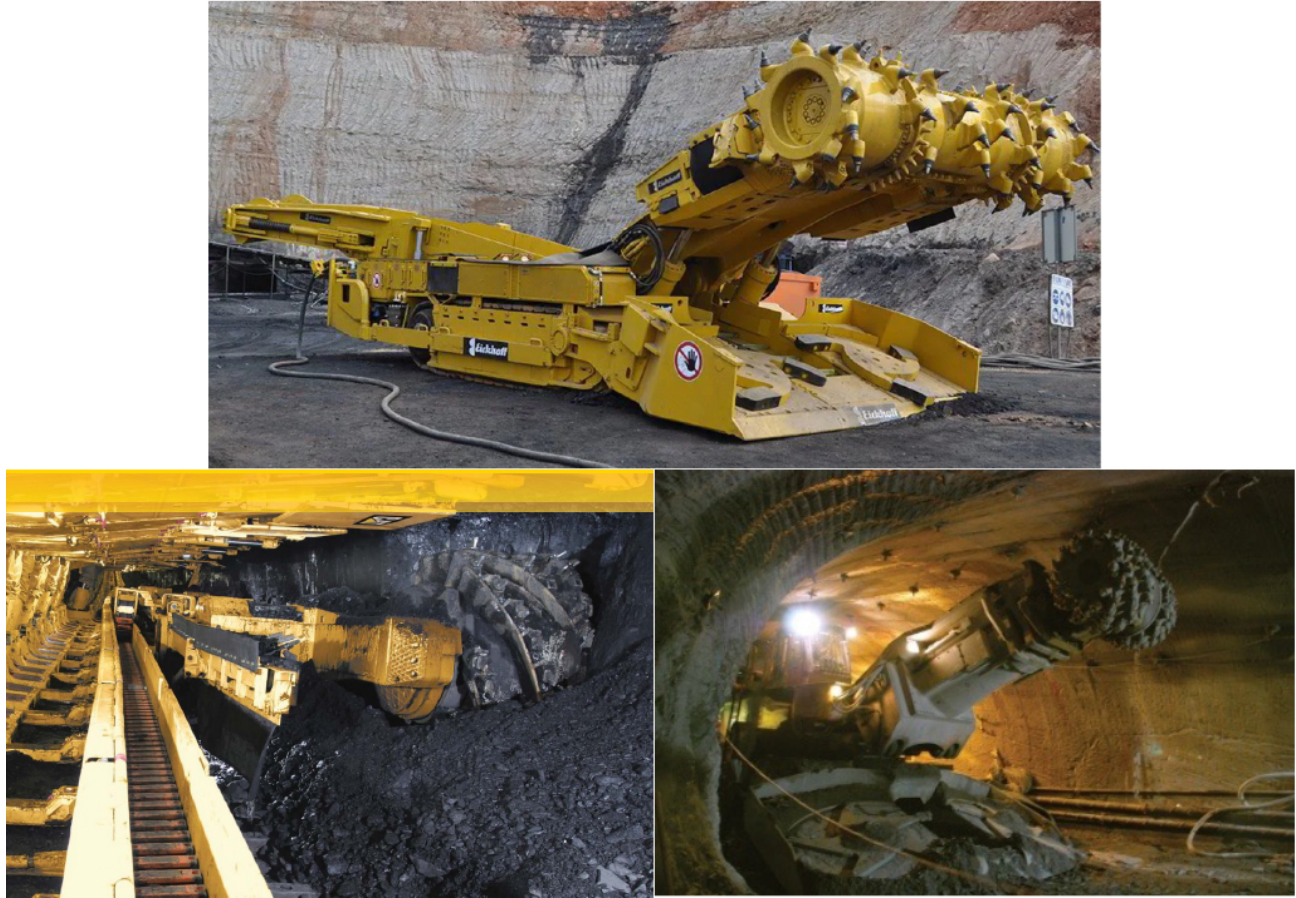
Figure 2: (Top to Bottom and Left to Right) Continuous Miner[2], A Longwall Shearer [3], Road Header [4].
