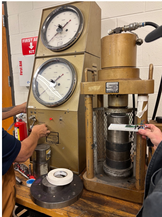
Figure 5 Hydraulic Press Experiment with Capacitive Load Cell.
