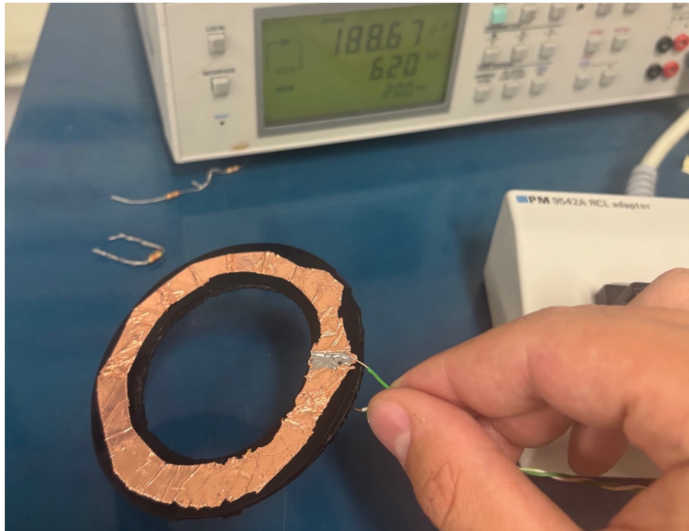
Figure 3 First Load Cell Used for Concept Exploration.
