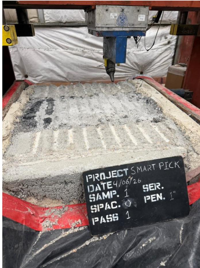
Figure 28 LCM With Integrated Load Cell
