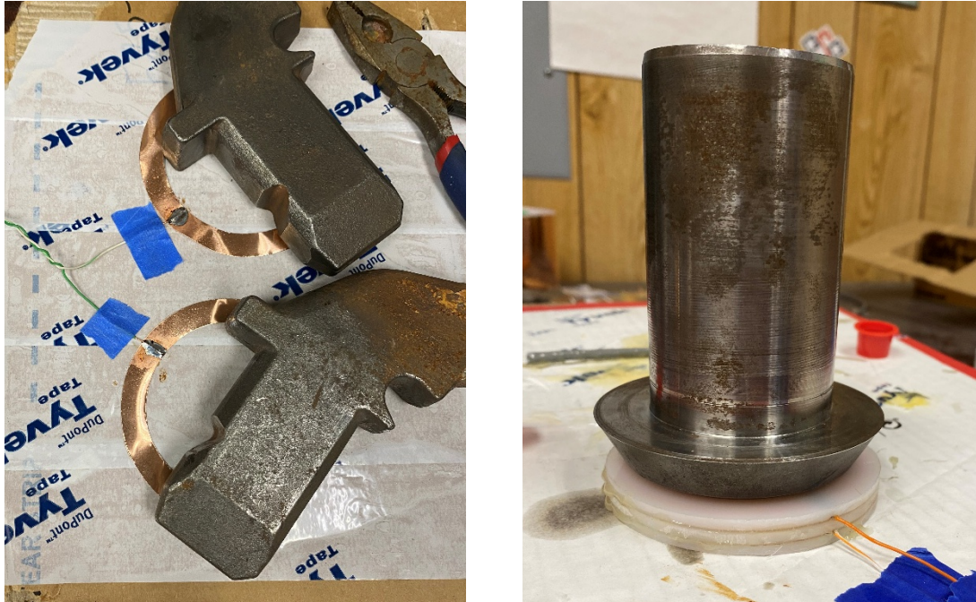
Figure 14: Prototype Assembly. Left: Soldering wires to copper. Right: Gluing layers together.
